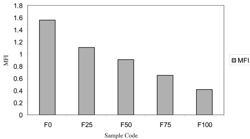
FIGURE 7. Effect of ATH loading on MFI of PP/EPDM blend
