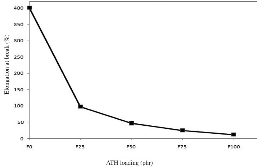
FIGURE 5. Effect of ATH loading on elongation at break of PP/EPDM blend
